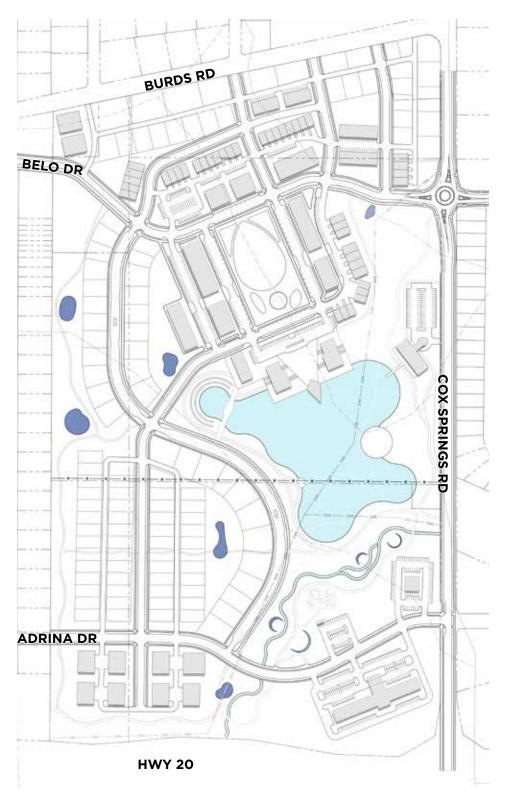
There is potential to develop a series of constructed wetlands, fourbays(?) and sediment traps in areas of the development to provide a low-impact approach to capture pollutants and slow runoff before water drains into the constructed wetland (Lake Peosta). Particular areas of consideration for stormwater management:
